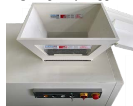
Figure 4: Safety cover for plane entrance and funnel entrance
