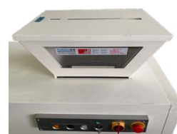
Figure 4: Safety cover for plane entrance and funnel entrance
